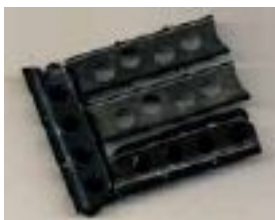
The Lee-Enfield bolt-action rifle was the main firearm used by the British and Commonwealth military from 1895 and is still in service in some countries. It uses a .303 cartridge, either loaded one round at a time or by using these five round chargers. During World War 1, contracts were placed with many of the Birmingham pen makers, including Baker & Fennimore, Perry & Co Ltd., M Myers and Sons and Brandauer. Contract prices were around four shillings per 100 or £2 per 1000.
