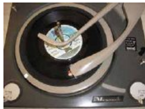
One of the very popular small Dansette record players, fitted with the widely used BSR Monarch deck
