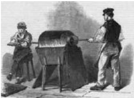
Bronzing, one of several processes for colouring pens
