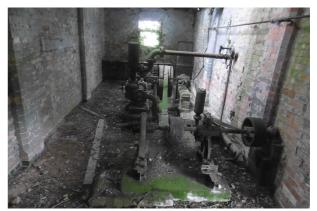
The machinery consists of a belt driven 'Tangye' single cylinder and double acting pump driven by a three phase motor by 'Higgs Motors of Witton' through a lay shaft and flat belting. The drive is clearly not original although the pump fits its base so well that it must be. The lay shaft has Wooden Pulleys and thus sits uncomfortably amongst the other machinery whilst a clutch is provided to slip the pump from the drive.
