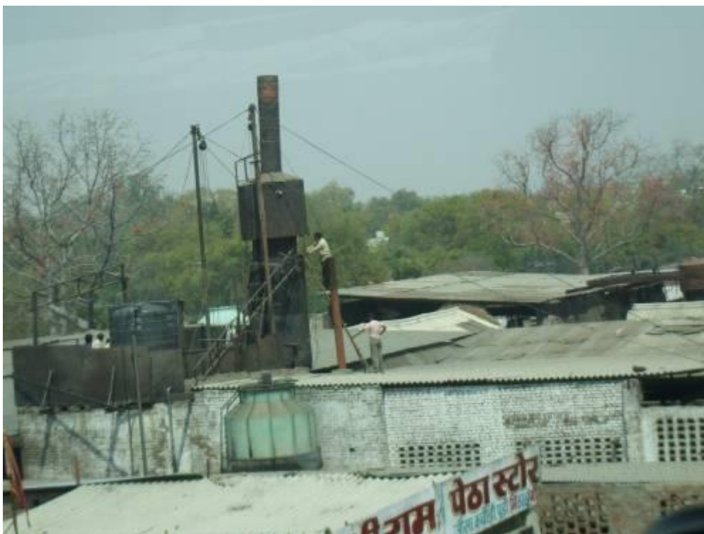
Top of a Cupola Furnace Stack in Delhi
